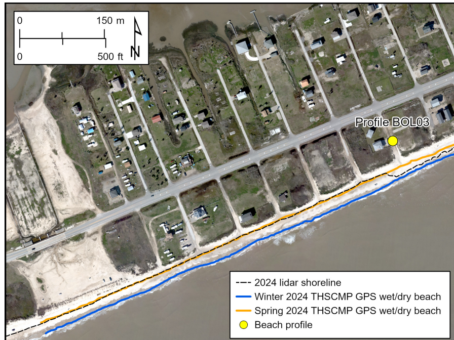
Figure 5. Shoreline position comparison at Bolivar Peninsula profile BOL03 near Rollover Pass (profile site BOL, fig. 4). Shorelines include the wet-beach/dry-beach boundaries mapped on February 1 (winter) and May 1, 2024 (spring) by THSCMP participants using ground GPS and the 1.16 m (3.8 ft) NAVD88 shoreline proxy extracted from the airborne lidar data acquired by the Bureau in 2024. The shorelines are superimposed on Bureau imagery that was collected concurrently with the lidar data.
