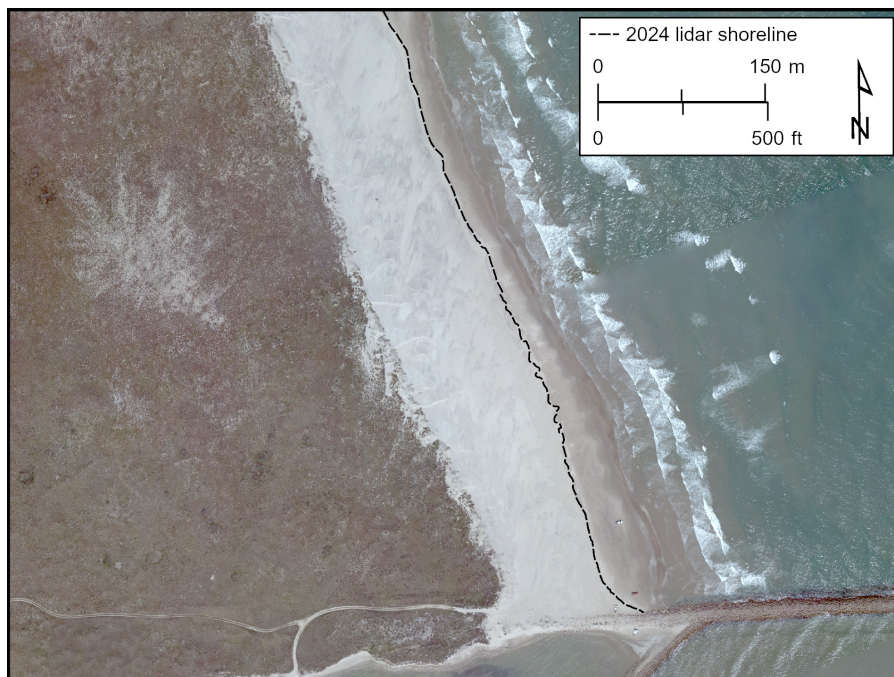
Figure 13. Shoreline position comparison on the lower Texas coast at Mansfield Pass (site MANP, fig. 4). The 1.16 m (3.8 ft) NAVD88 shoreline proxy extracted from the lidar data is superimposed on 2024 Bureau imagery.
