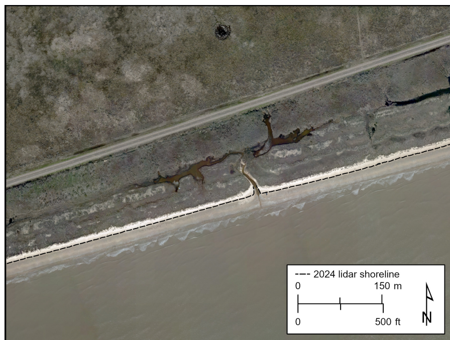
Figure 11. Shoreline position comparison on the upper Texas coast at Sea Rim State Park (SRSP, fig. 4). The 1.16 m (3.8 ft) NAVD88 shoreline proxy extracted from the lidar data is superimposed on 2024 Bureau imagery.
