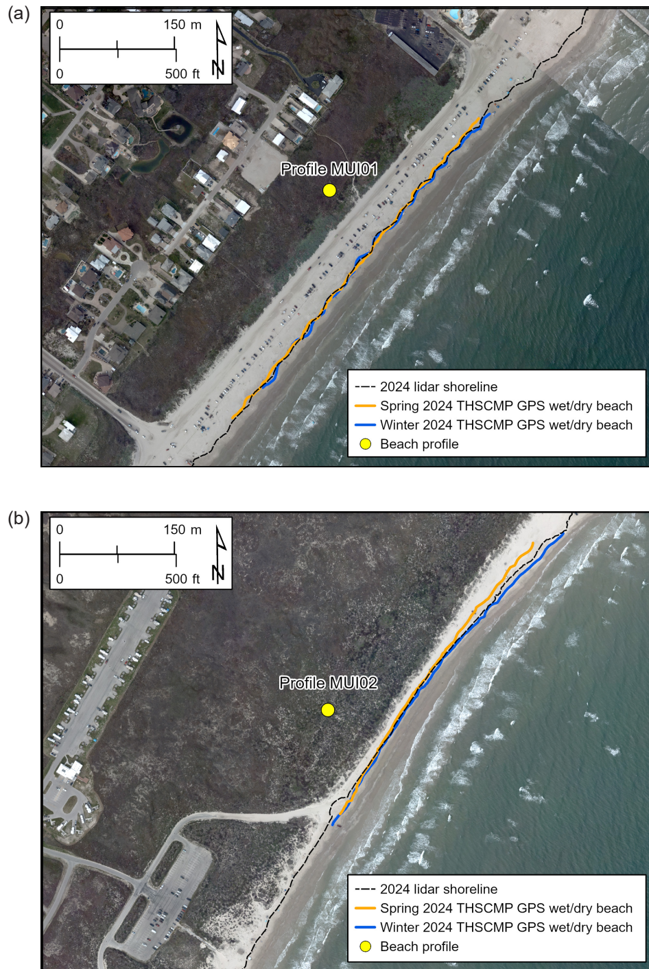
Figure 9. Shoreline position comparison at Mustang Island sites (a) MUI01 and (b) MUI02 (fig. 4). Shorelines include the wet-beach/dry-beach boundaries mapped on February 22 (winter) and April 25, 2024 (spring) by THSCMP participants using ground GPS and the 1.16 m (3.8 ft) NAVD88 shoreline proxy extracted from the lidar data superimposed on the 2024 Bureau imagery.
