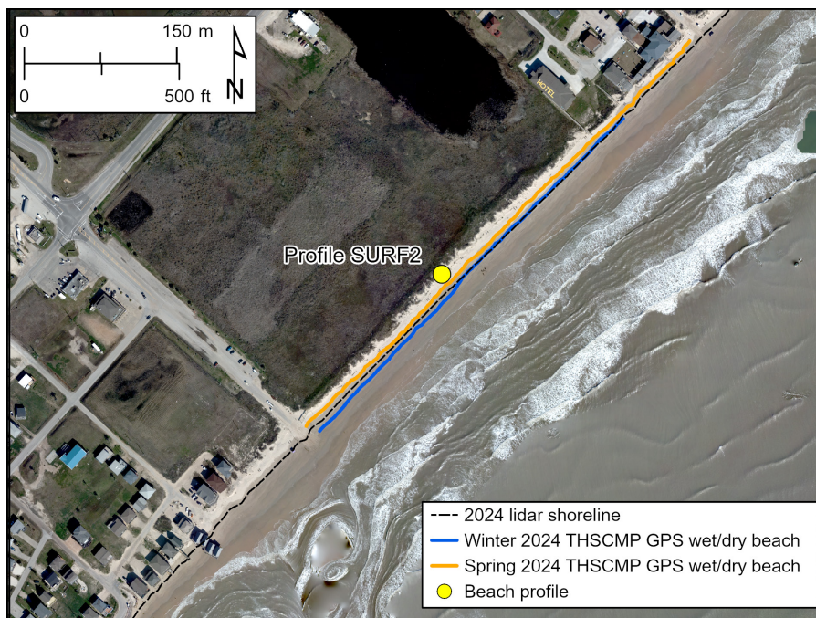
Figure 7. Shoreline position comparison at Surfside Beach site SURF2 (profile site SURF, fig. 4). Shorelines include the wet-beach/dry-beach boundaries mapped on January 19 (winter) and May 3, 2024 (spring) by THSCMP participants using ground GPS and the 1.16 m (3.8 ft) NAVD88 shoreline proxy extracted from the lidar data superimposed on the 2024 Bureau imagery.
